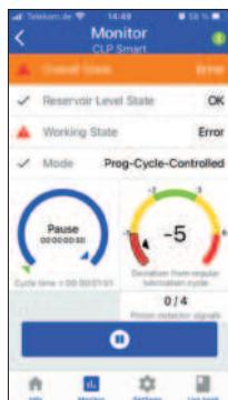
When accessing the monitor screen, users have at all time the possibility to initiate an additional lubrication cycle to check pump functionality.
