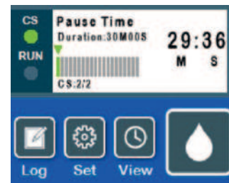
Pause time, shown in active mode, where users can interact with the pump
